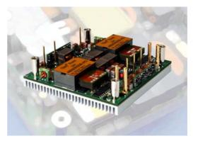
Buck-Reset topology it is demonstrated with the unique single board single side component structure. The integrated Sink-Plate design also helps the power module to get the best thermal performance and to deliver high power under extreme environmental conditions.
